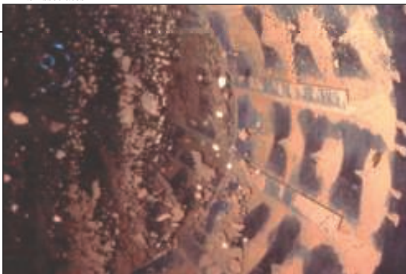
FIGURE 2. This photo shows how flights lift and drop sand through the hot gas stream in a rotary dryer
