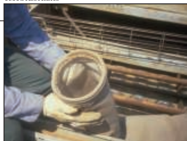
FIGURE 5. Shown here is a filter bag with cages and blow pipes in the background
